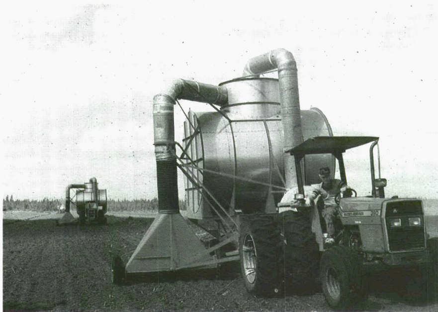
Tractor-drawn vacuum machines are used to harvest dried peat from production areas across Canada.
